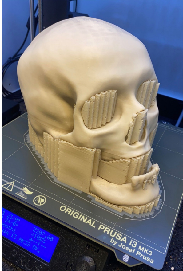
Figure 4: 3D printing humans: This 3D printed skull is a reconstruction of a real medical imaging dataset. Students do not only learn theory; they finally have a tactile result of their learning success.
