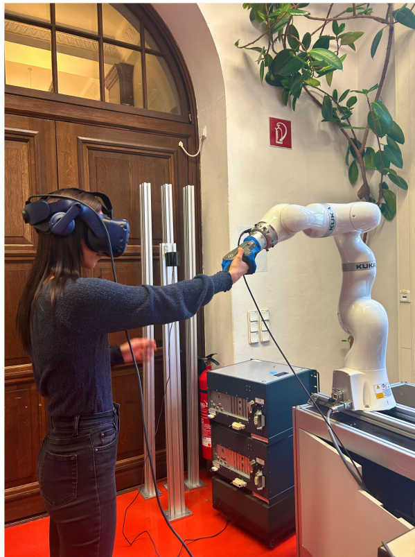
Figure 1: Human-Machine Interaction via Virtual Reality. The intelligent robot is controlled by gestures, hand controllers or Virtual Reality gloves, a bunch of sensors, cameras and artificial intelligence. (Hanshans, CC-BY-SA-NC)
